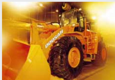
Simulation of extreme weather conditions (cold, warm and wet weather).
