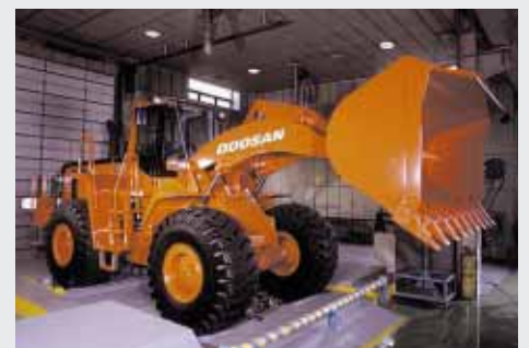
Rolling conditions simulations (braking, acceleration, drawbar pull, heat dissipation ...).
